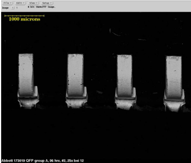
Figure 4. Group 2A NiPdAu 0.02- \mu\text{m} (0.8- \mu\text{”} ) Pd, Loose, 96 h, 25 \times
